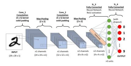
Figure: Convolutional neural network architecture.
